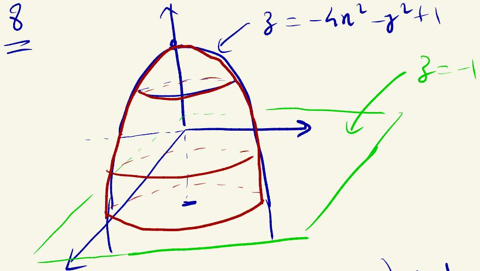
$$\text{Vol} = \iint_D \left( 4x^2 + y^2 + 1 - (-1) \right) dx dy$$
